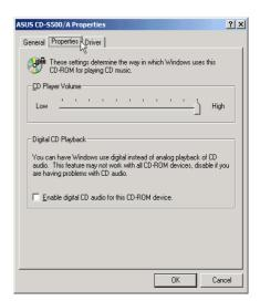
Figure 2-6: Enabling Digital CD Audio in Windows 2000
